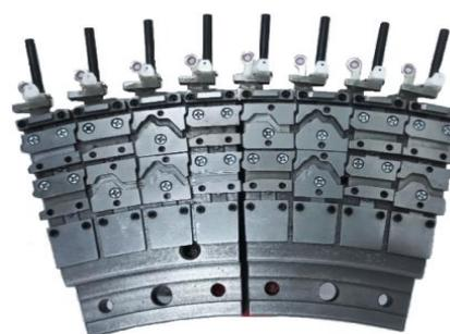
**Figure 3.** - The weaving system of the circular two-needle knitting machine
