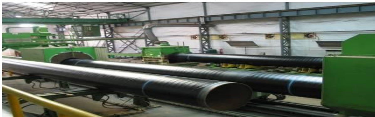
Figure 2. External Anticorrosive layered pipes
